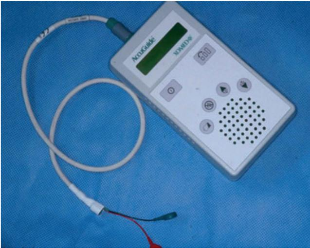
**Figure 4** Pocket-sized EMG machine used for injection guidance
